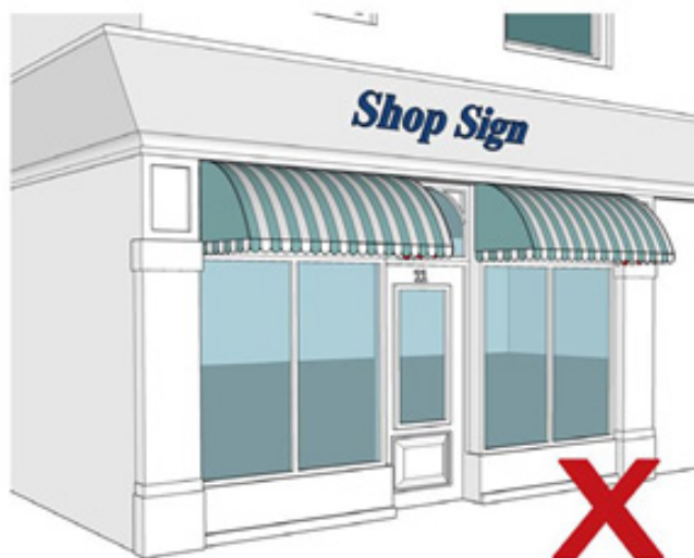
Non-retractable Dutch blinds should not be used
