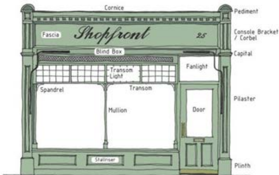
Typical traditional shopfront with architectural features labelled
